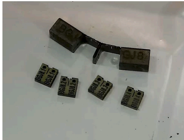
Fig. A1. Extracted C(T) specimens from a Charpy sized specimen.
