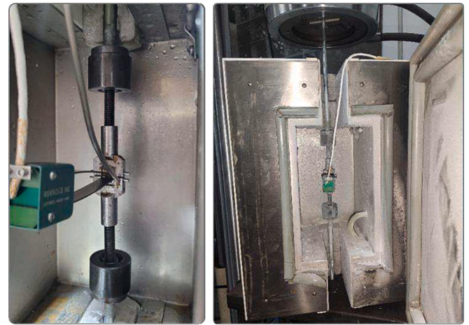
Fig. 3. Experimental setup of the mini-CT specimen.
