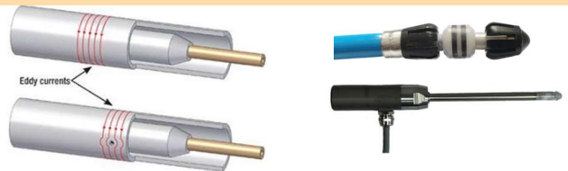
Fig. 1 Principle of ECT and typical Bobbin probe design and High speed Motorized Rotating Pancake Coil probe.
