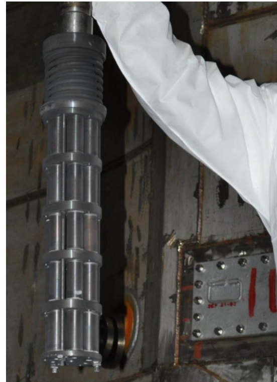
WWER-1000 surveillance assembly for thermal ageing monitoring
